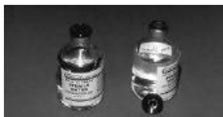
The water vials. On the left as used in the sessions, on the right cap seal off showing rubber seal through which needles were inserted.
